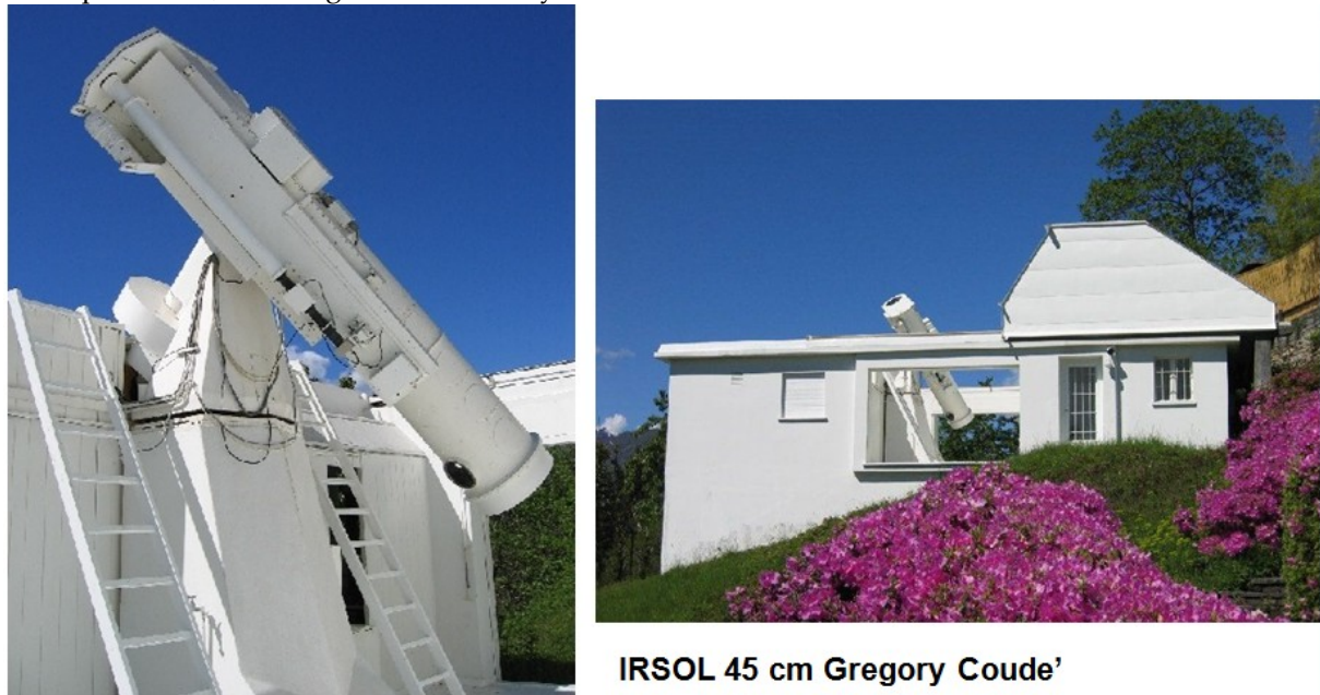
Fig. 4.8 The Gregory-Coudé solar telescope at IRSOL, 500 m above sea level, and 300 above the Maggiore lake. This instrument benefits of very good seeing.
