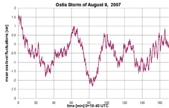
FIGURE 13. Data obtained during a sea storm 100 m inside the fishermen's canal-port of Ostia (Tyrrhenian sea). 4 minutes edge waves disturbances are visible superimposed to main seiches of 30-40 minutes periods. Open sea waves of 2 m height were measured during that storm. Running average on 8 minutes and tidal trend averaged on 25 minutes subtracted; other combinations of averages show similar patterns. Waves direction was from SW, and the canal is oriented toward South. The canal depth is h=1.4 m and its width 15 m. With wavelengths \lambda=21.7 \pm 0.9 m and periods of 6.7 \pm 0.9 s the waves, in this canal, propagate in shallow water regime at a speed v=3.24 \pm 0.57 m/s. Shallow water speed for this canal is v=\sqrt{gh}=3.70 m/s. The effect of wave setup which modulates the 20 to 40 minutes seiches with 4 minutes fluctuations is efficient even inside the canal.
