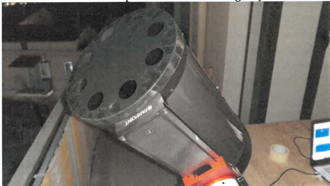
Fig. f a C9 telescope (28 cm) masked with eitght-4cm holes.
